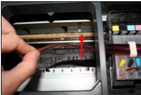
Circumrotate the tube 90 degree as above picture shown.
