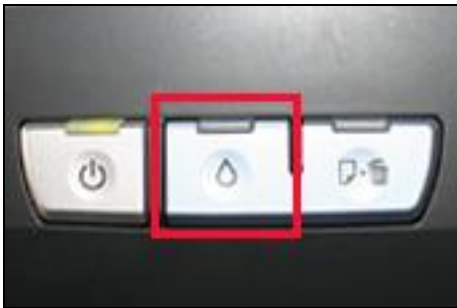
Press the button to replace cartridges
