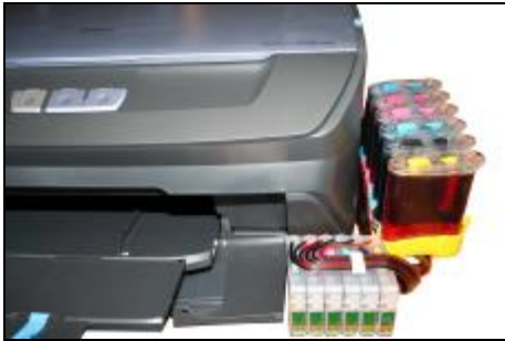
Put the CISS on the left side of the printer. and place all the tubes at correct position.
