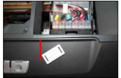
Stick the other clip on left button side of the printer, the angle is 30 degree
