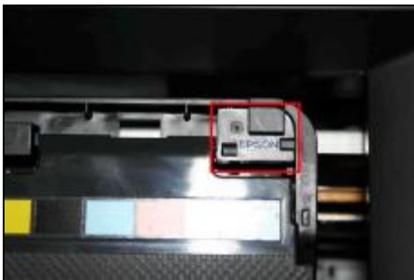
Remove the clip of the cartridge, as the above red rectangle shown.
